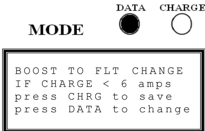
This changes the charge current at which the BOOST mode after timing out changes to FLOAT. This can be 3 – 6 – 15 - 30 amps or Disabled. Press <CHARGE> to save. The screen will then change to:
