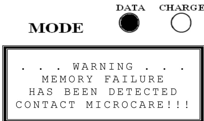
The Internal PIC (Memory Chip) in the MPPT is becoming full and is starting to detect that it is full. This warning can be overcome by restarting the MPPT, however the problem will start occurring more often.
