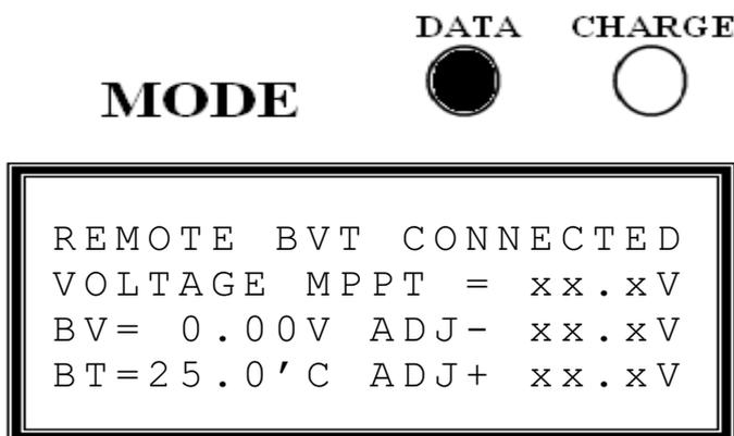
This shows the battery temperature and voltage. Should there be a problem with the cable or a poor connection then the screen will flash ERROR.
