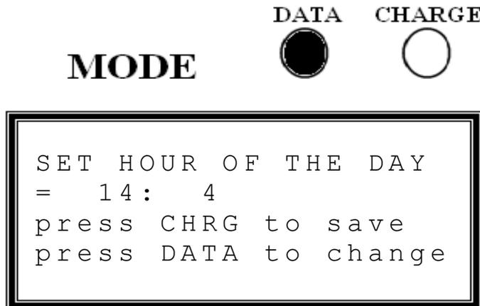
This allows the user to change the time settings of the MPPT. The Hour of the day is changed in this screen through a 24hour time format with 1 hour increments. By pressing the <DATA> button, the display will then change to change the minute's settings of the MPPT:
