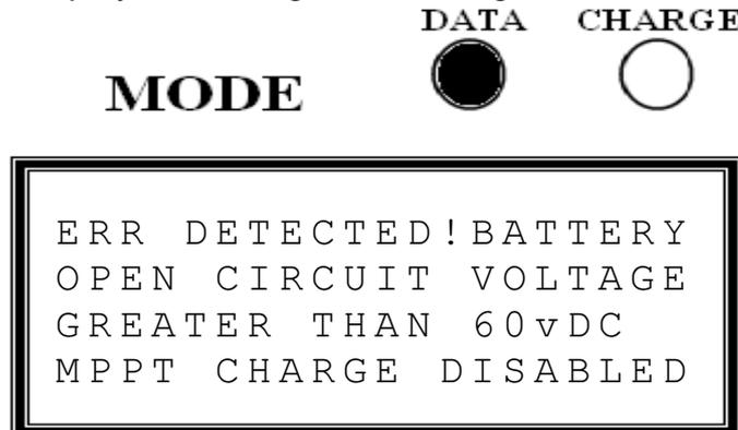
The Battery Voltage is exceeding the supported Voltage range of the MPPT.
