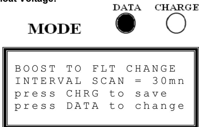
This screen changes the time that the BOOST mode takes to switch to FLOAT mode once the batteries have reached the BOOST voltage level. The time can be 30minutes – 1 hour – 2 hours. Press <CHARGE> to save. The screen will then change to:
