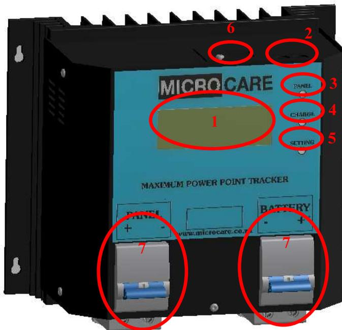
1. LCD Display: This indicates the MPPT's operation including Panel voltage, charge condition, charge amps, battery voltage and output power.
