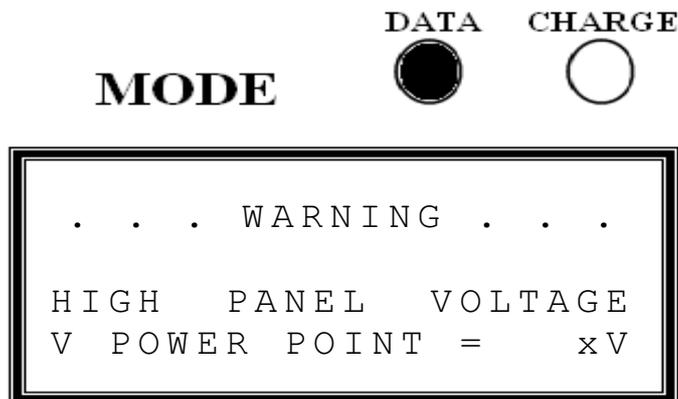
This error will display when the PV Voltage is exceeding the 4:1 Ratio between the battery voltage and the PV Panel Voltage used to charge the batteries.
