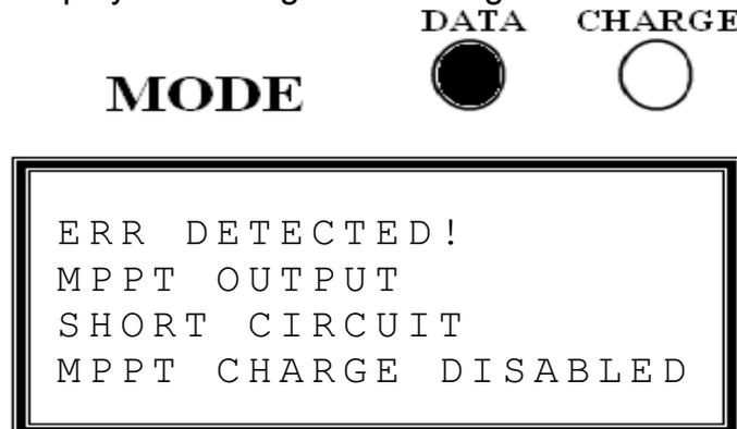
This error message will be displayed if the load being drawn from the batteries is exceeding the amount of power that the MPPT is capable of supplying.
