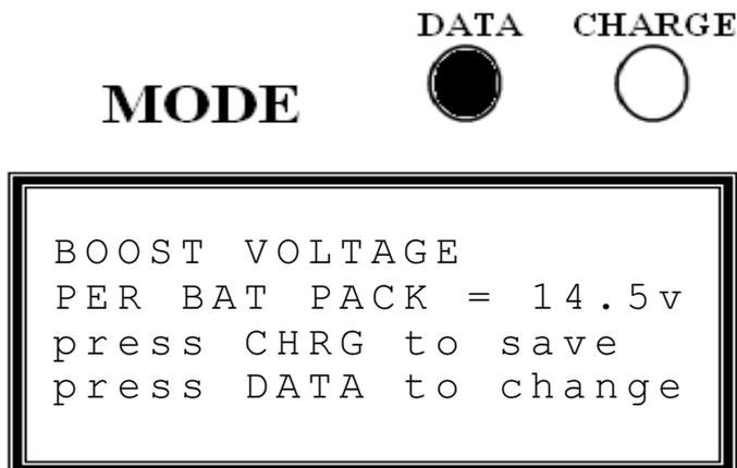
The Boost voltage can be changed between 13.5 and 16.0 volts with 0.1 volt increments. Press <CHARGE> to save. The screen will now change to:
