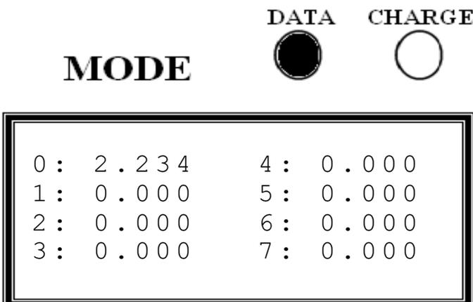
This shows the energy accumulated since the charger started. The 24Hr is the daily average for the no of days shown. Should you wish to CLEAR the DATA then hold the **<CHARGE>** button in for 6 seconds and the values will reset to 0.
