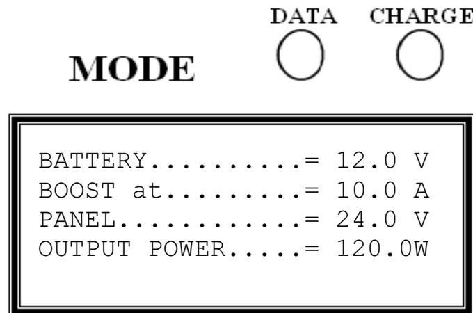
This is the screen that will normally be displayed showing the system operating correctly. There are other details that will appear on the screen that will assist the user to read at what point the MPPT and batteries are:
