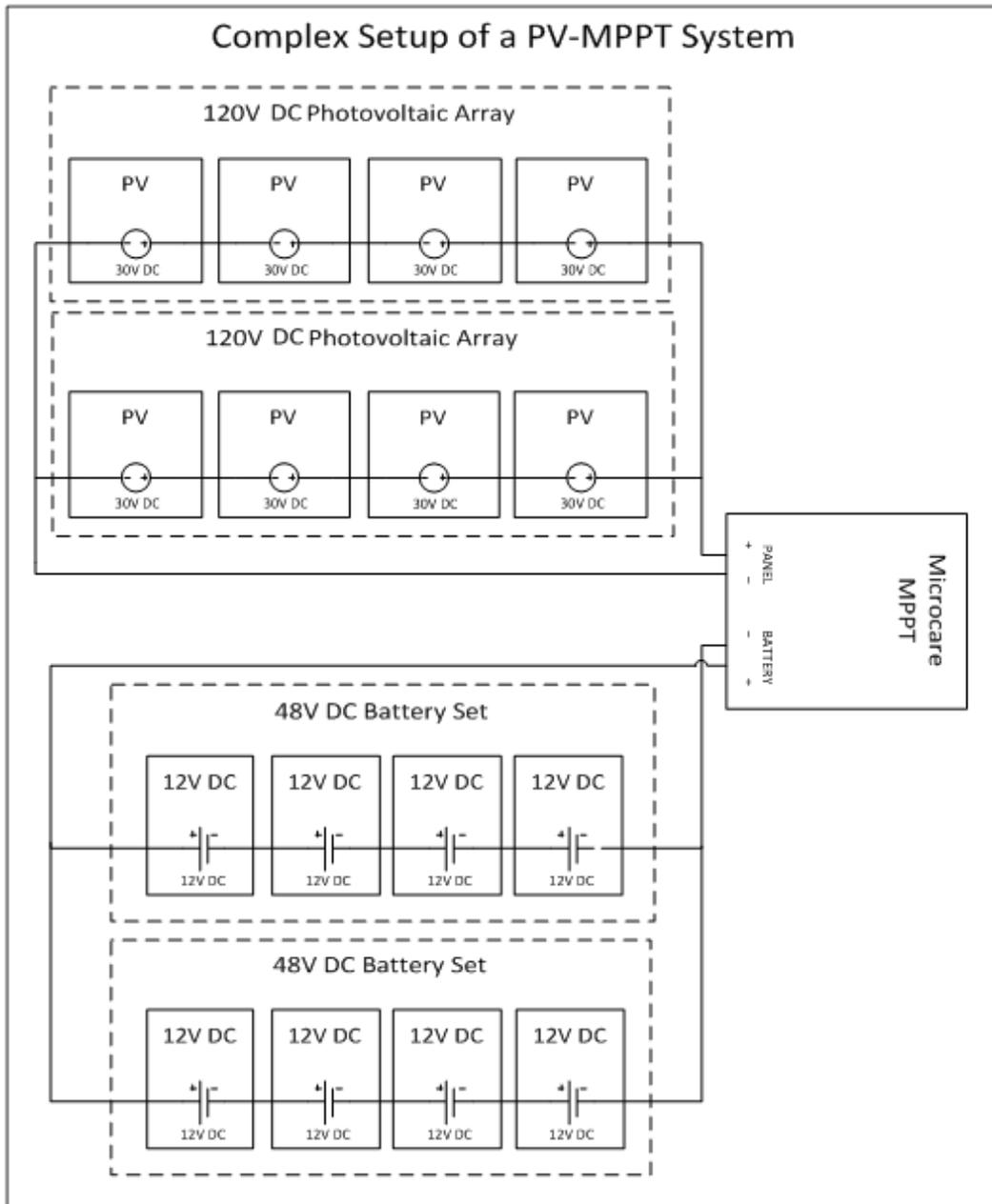
A complex PV-MPPT setup can have arrayed PV and Battery Sets all connected in parallel. The voltage of the PV array may not exceed 150V and depending on the MPPT model, a specified current strength. The Battery Set array is however unlimited in size although an increase in Battery Set array length will increase the amount of time needed to fully charge the batteries.
