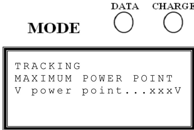
This shows the MPPT measuring the open circuit panel voltage and calculating the initial power point voltage.
