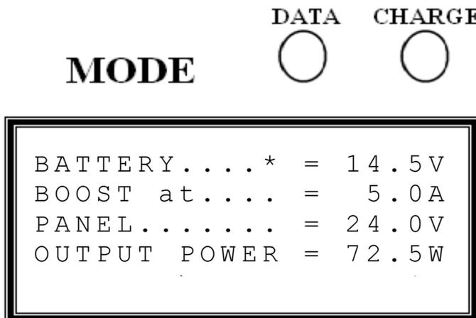
When the charge current falls below the programmed value of say 5.0 amps, the screen will then change to:
