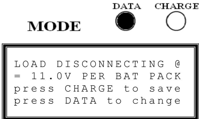
The user can program the Voltage at which the RELAY operates. This is between 10-12 volts per pack, in 0.1 volt steps. If the system is 48 volts multiply the settings by 4.
