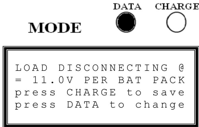
The user can program the Voltage at which the RELAY operates. This is between 10-12 volts per pack and increments in steps of 0.1 volts. If the system is 48 volts, multiply the settings by 4. If this is complete then the LOAD SHED RECONNECT voltage can be programmed which can be between 12-14 volts per pack:
