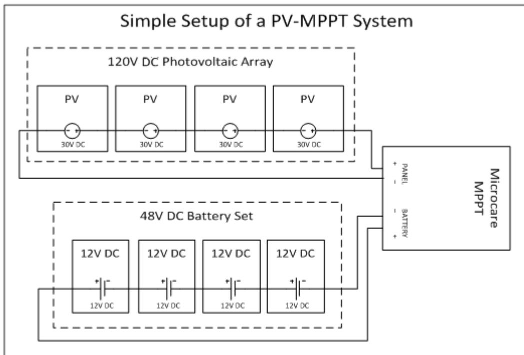
A simple PV system setup is illustrated with 48V DC Battery Set.
