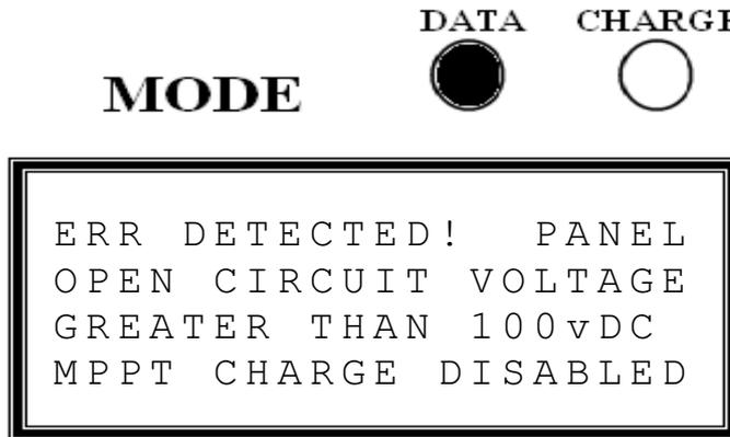
Your PV Panel array is connected in series and is exceeding the 150Voc capacity of the MPPT
