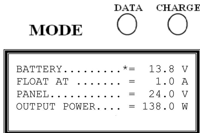
The \* flashing next to the batteries indicates that the MPPT is in FLOAT mode and the batteries are full.
