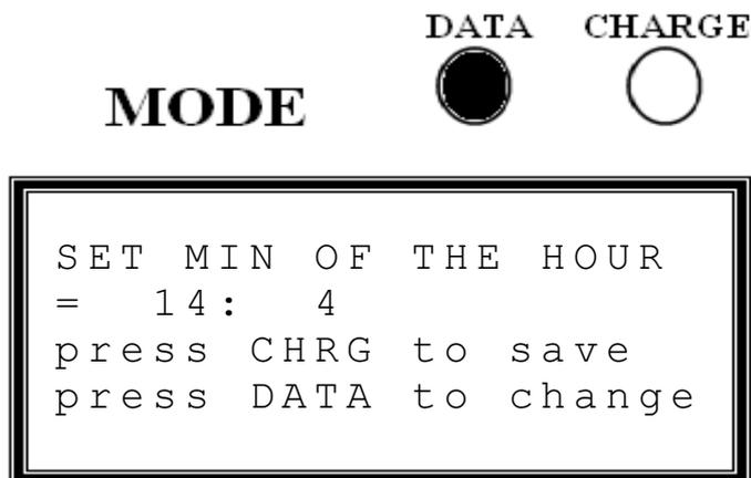
In this screen, the clock's minutes are adjusted in a similar fashion to that of the hour settings. Pressing the <DATA> button again will exit the settings menu and the MPPT will then reset itself with all adjusted settings loaded and normal MPPT operation will continue as soon as the PANEL breaker is reset.
