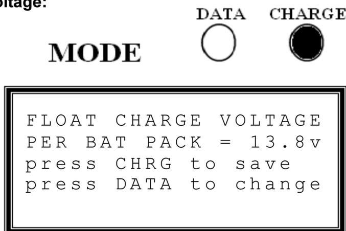
To change the battery pack FLOAT VOLTAGE push the **<DATA>** button and the voltage can be changed from 13.2 to 14.5 volts with 0.1 volt increments.
