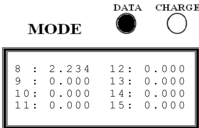
Day 0 shows the power accumulated for the current day. Up to 31 days of data is stored and may be viewed by pushing the **<DATA>** button. To clear the screen, hold in the **<CHARGE>** button in for 10 seconds or until the data has been cleared.
