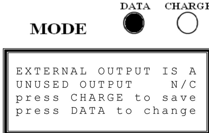
Pushing the **<CHARGE>** button will change the external output from being an UNUSED output to a:
